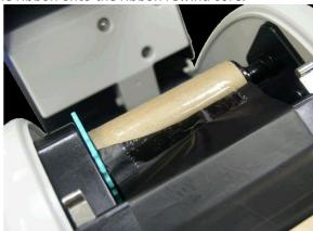
6. Turn the ribbon rewind gear until the ribbon plastic leader is thoroughly wound and the black section of the ribbon covers the print head.
