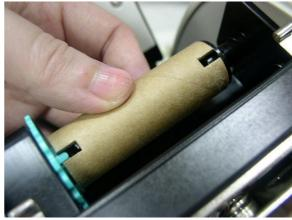
5. Pull the leading ribbon to pass the print head. Stick the ribbon onto the ribbon rewind core.
